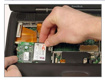
Use the tips of your fingers, a spudger, or a flat non-metal tool to get under the modem's edge and pry it up from its socket.
