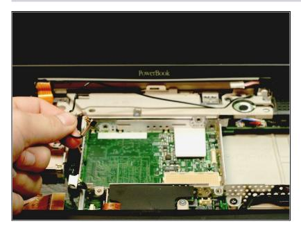
• Returning to the front, pull the black Airport antenna up from its recessed housing.
