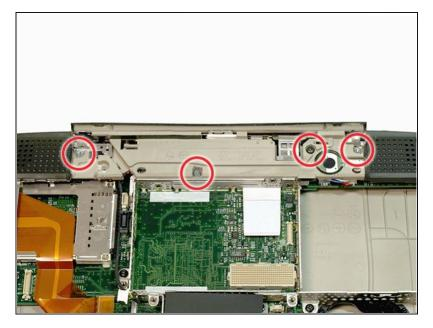
Remove the three long silver and one short black Torx screws from the beige plastic casing.
