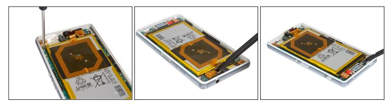
• Release connectors and twist off screw.
