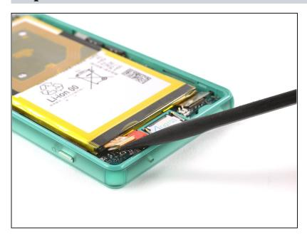
Disconnect the battery flex cable.
