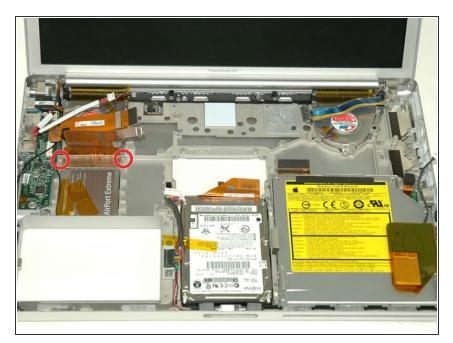
Remove the two silver Phillips screws from either side of the large orange Airport ribbon.
