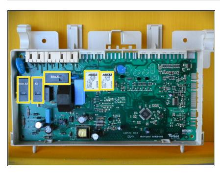
There are three or five relays on the circuit board. K6 is an OMRON G2RL-1A-E, 12VDC, and rated to switch 16A at 250 VAC. K1 and K4 are both OMRON G5LE-1-VD, 12 VDC, and rated to switch 10A at 250 VAC.
