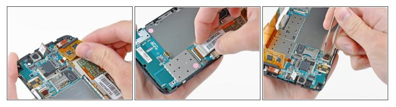
• Before lifting out the motherboard, the touchscreen, LCD, and control button ribbon cables must be disconnected.
