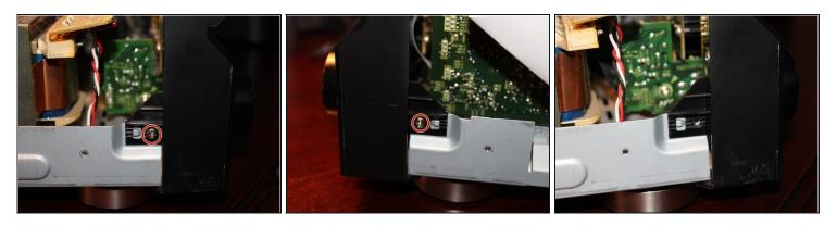
• After the faceplate pin is removed, remove the 2 screws that hold it to the chassis. Both screws are the same length.
