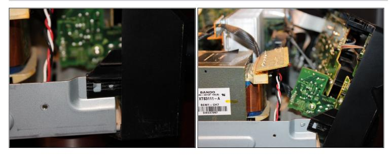
⚠ Once the unit is reassembled, these zipties must be replaced. Failure to do this will result in protection mode errors.
