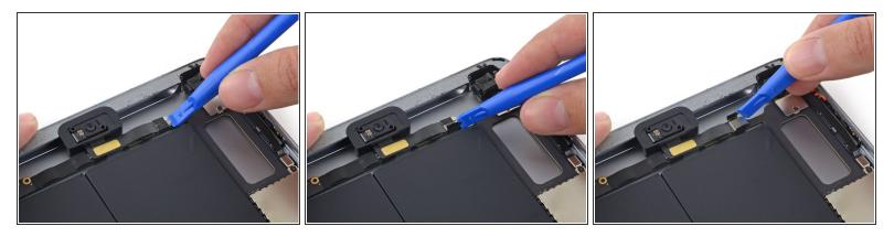
Use a plastic opening tool to fold the front-facing camera cable clips outward, away from the cable, freeing the cable connector.
