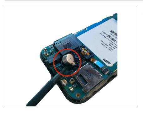
Using a spudger/pry tool, carefully remove the vibration motor from its housing. This has a mild adhesive on the bottom.
