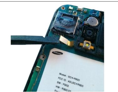
Using your spudger/plastic pry tool, disconnect the rear speaker flex cable.
