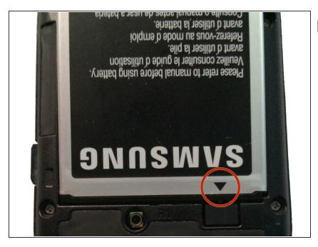
Make sure when replacing the battery that the arrow on the bottom is facing down.
