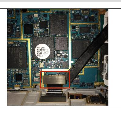
Using your spudger/plastic pry tool, disconnect the LCD/Digitizer flex cable.
