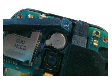
• Using your spudger/plastic pry tool, disconnect the headphone jack flex cable.
