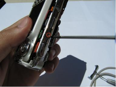
Remove the top panel screw (1x 4.37mm).
