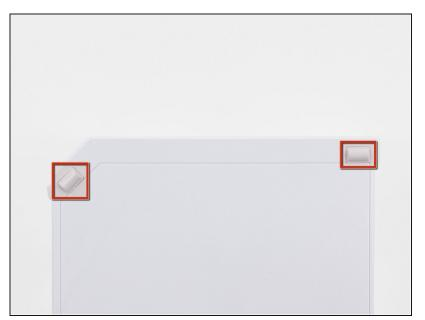
Use a metal spudger to remove the two rubber feet stuck to the bottom face of the Wii near the rear ports.
