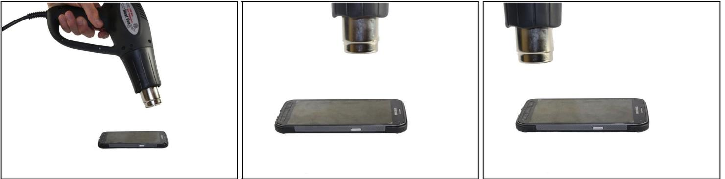
☑ Make sure the battery, the SIM card, and the MicroSD card have been removed. If these components are not removed, they may get damaged when the heat is applied.
