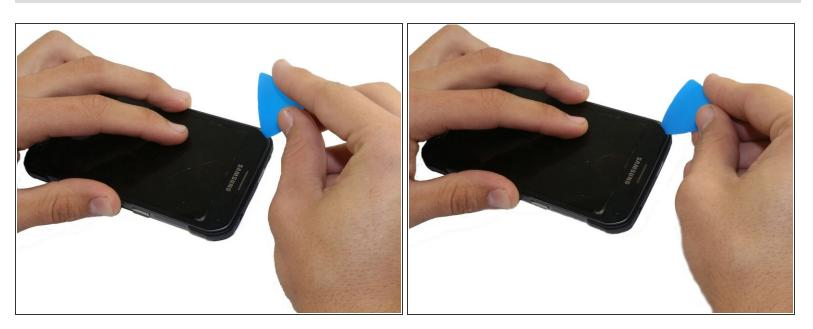
Starting from the upper left corner, insert a guitar pick in between the display and the phone case.
