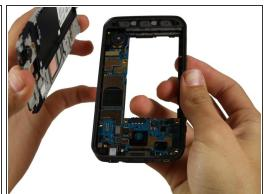
Push upward from the back side your phone (where the battery should go) to pop out the large gray piece.
