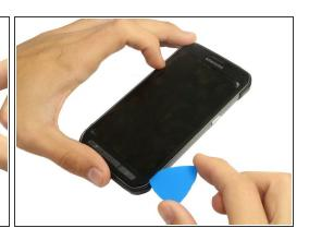
• Use the pick to pry the sides and lower part of the display by sliding the pick through the phone.
