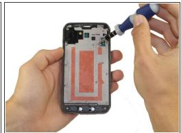
Use a Phillips 0 screwdriver to remove all 12 Phillips #0 screws.
