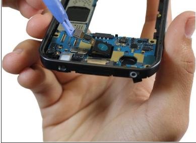
Use your finger or a plastic opening tool to disconnect the rear-facing camera from the motherboard.
