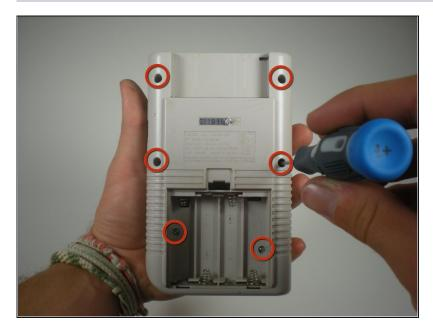
• Remove the six Triwing screws from the back of the device.
