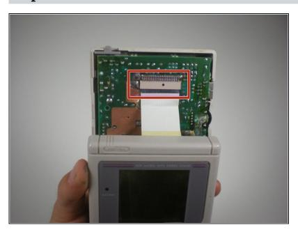
Slide the front side of the casing down to expose the ribbon cable connector.
