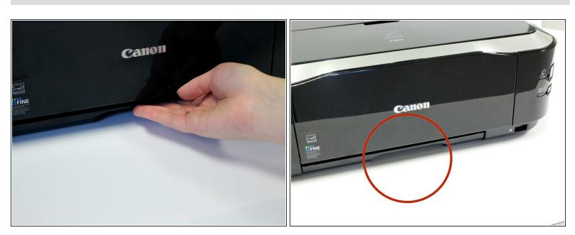
• Reach underneath printer, fitting your fingers into the groove in the front of the cassette.
