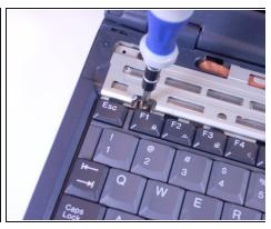
• Using an Phillips screwdriver, unscrew and remove two screws labeled B2.6.
