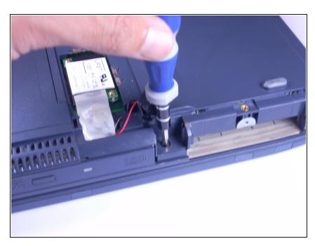
Using a Phillips screwdriver, unscrew and remove one F6 screw from beneath the modem.
