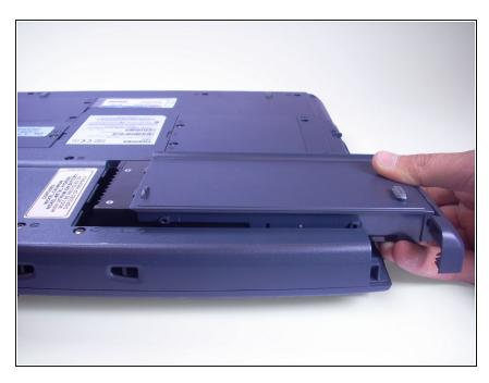
• Lift the battery casing out of the laptop.
