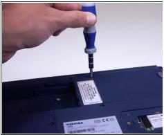
Using a Phillips screwdriver, unscrew and remove 3 B25 screws from the bottom of the laptop.
