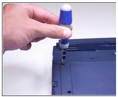
• Using a Phillips screwdriver, unscrew and remove 3 F6 screws from the bottom of the laptop.
