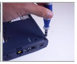
Using a Phillips screwdriver, unscrew and remove 5 B20 screws, located along the corners of the bottom of the laptop.
