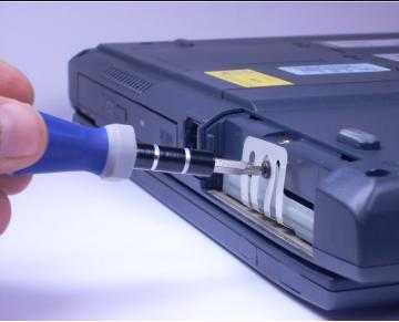
• Using a Phillips screwdriver, unscrew and remove the screw surrounded by the white plastic.
