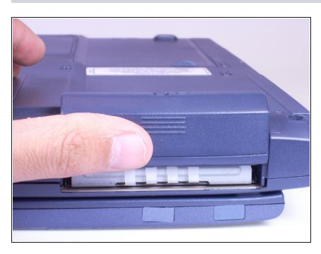
Placing your finger on the raised grip, push up on the hard drive cover. This will remove the hard drive cover from the laptop.
