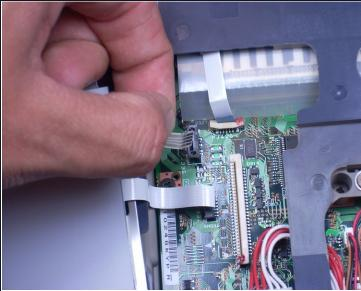
Remove the left, brown ribbon by pinching the part of the ribbon connected to the computer and lifting towards you.
