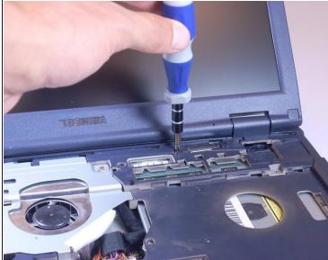
• Using a Phillips screwdriver, unscrew and remove two screws labeled B25 located closest to the screen.
