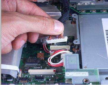
Setting screen next to the base of the laptop, pinch the connecting cable with your fingers and gently pull connecting cable from monitor. To reassemble your device, follow these instructions in reverse order.
