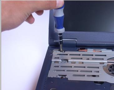
• Using a Phillips screwdriver, unscrew and remove 5 screws labeled F6, located on the metal piece on the left side of the keyboard area.
