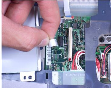
Remove the white ribbon on the right by pinching the part connected to the laptop with your fingers and pulling towards you.
