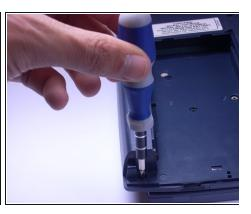
Using a Phillips screwdriver, unscrew and remove 3 F4 screws from the battery area of the laptop.
