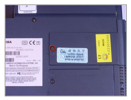
Using a Phillips screwdriver, unscrew and remove F4 screw from plastic covering on the bottom of the laptop that only has one screw.
