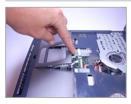
Using your finger, lift off the plastic covering the trackpad by putting your finger underneath the plastic and pulling towards you. The plastic should just pop off.
