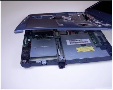
• Lift open the screen of the laptop and, using your fingers and the guides on the side of the laptop, push up on the top plastic covering of the laptop, moving from one side of the laptop to the other.
