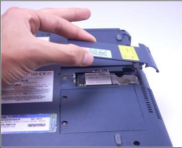
• Using fingers, pinch and lift plastic covering up, away from the laptop and set aside.
