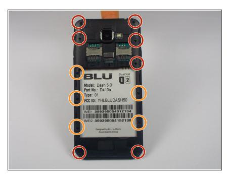
Using the PH00 Phillips head screwdriver unscrew the screws holding the panel down, making sure
