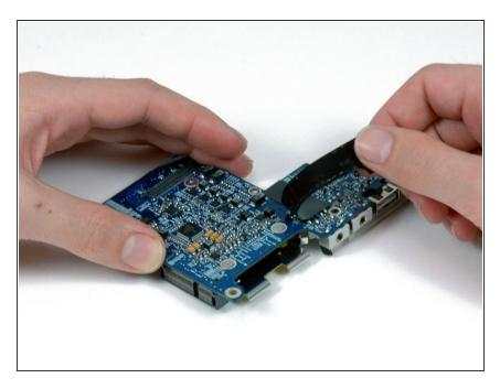
Peel up the L-shaped piece of black tape on the I/O board to reveal the two silver Phillips screws beneath.
