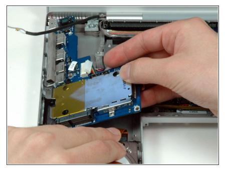
• Move the orange hard drive ribbon out of the way with one hand. Use your other hand to lift up the right side of the left I/O board and slide it out of the computer.
