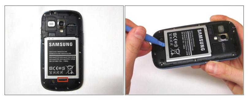
• Use your finger or an opening tool to pry the battery out of the phone.
