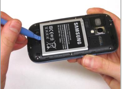
Use your finger or an opening tool to pry the battery out of the phone.
