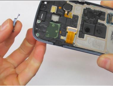
The power button is connected by two plastic posts, simply lift the button away from the phone using your fingers.
