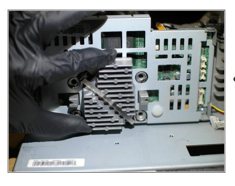
while reassembly is generally the reverse of the dis-assembly, when re-installing the heatsink you should make sure it's a snug fit once the clip is installed. Wiggle the heatsink; it should move very little. If it moves too much, remove the clip and bend the ends upward so that it provides more tension when it is installed.
