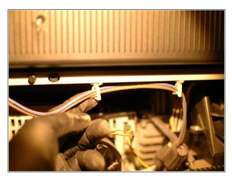
While not completely necessary, it can help to remove this power cable from the cable ties that hold it to the top of the TV frame. This will get it out of the way when you remove and install the light engine.
