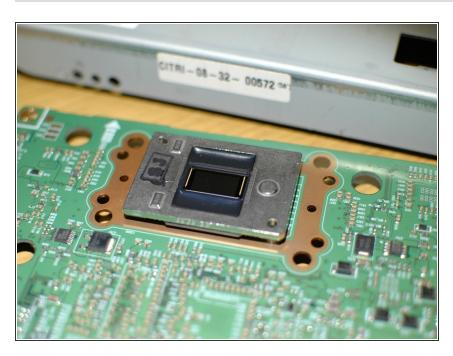
Here is the new DLP chip, and so we are ready to reassemble!
