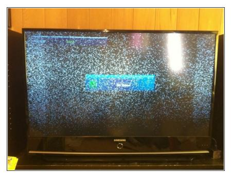
Here is a prime example of a failed DLP chip. The TV has become basically impossible to use due to the overwhelming number of stuck mirrors in the DLP chip. Let's fix it!
