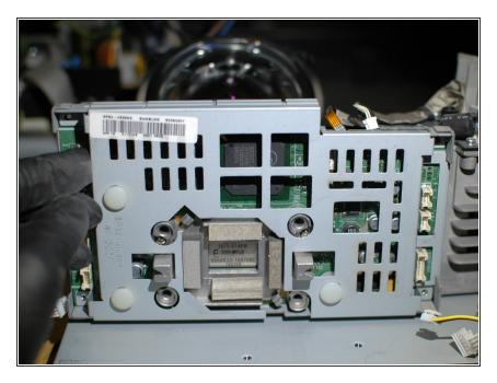
Then remove the outer DMD board cover by pulling it away from the board gently.
