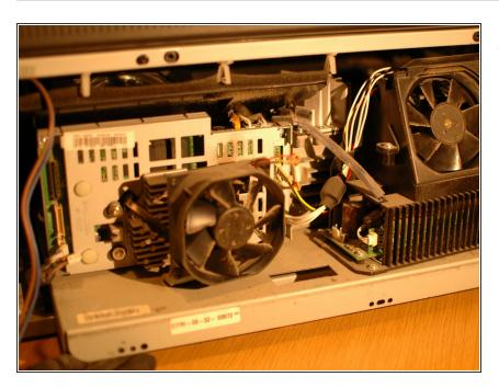
Now you can pull the light engine out of the body of the TV by pulling it straight out. It rides along rails in the TV frame and should slide straight out, though you may need to lift it over a few bumps along the way.
