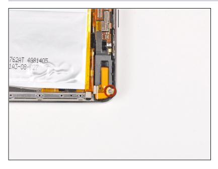
Remove the remaining Phillips screw securing the upper logic board to the rear panel.
