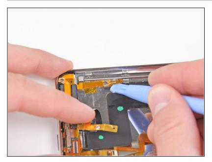
Use the edge of an iPod opening tool to peel the antenna socket ribbon cable off the rear panel.
