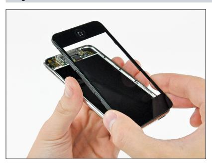
Lift the front panel out of the rear case minding the cable still attaching it near the upper left corner of the Touch.
