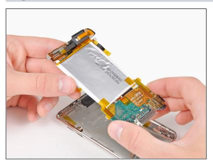
Carefully remove the logic board assembly from the rear panel, minding any cables that may get caught.
