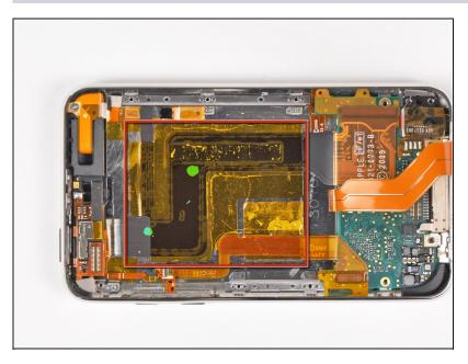
Carefully remove the two large pieces of tape securing the ribbon cables to the rear panel.
