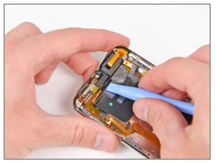
Use an iPod opening tool to pry the black plastic frame under the upper logic board up from the adhesive securing it to the rear panel.
