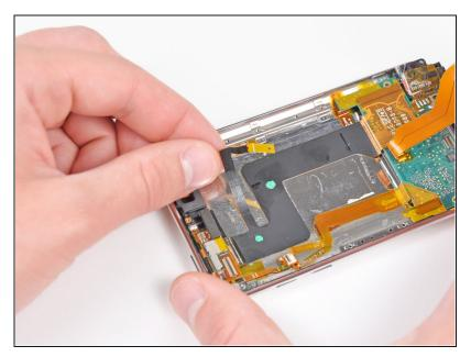
Carefully peel the antenna cable off the adhesive securing it to the rear panel.
