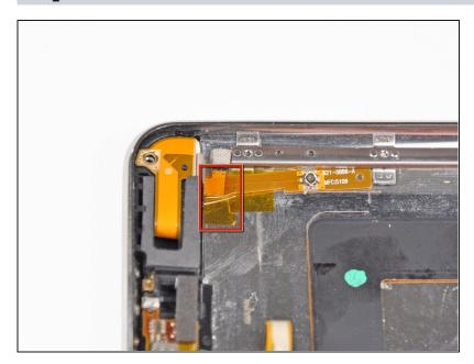
Remove the small strip of tape securing the antenna socket ribbon cable to the rear panel.
