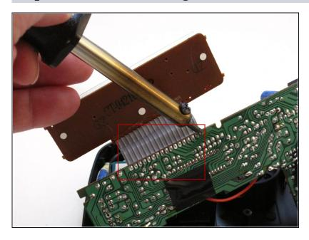
Carefully apply the heated soldering iron on each of the 17 ribbon cable pin solders (first one as shown). Continue until the ribbon cable is detached.
