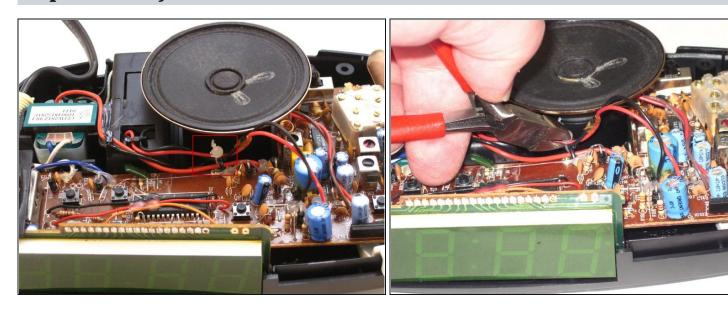
• Using the wire cutters, carefully cut the plastic wire tie.
