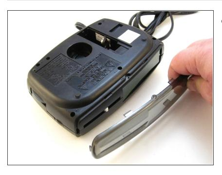
Gently pull the liquid crystal display (LCD) cover off.
