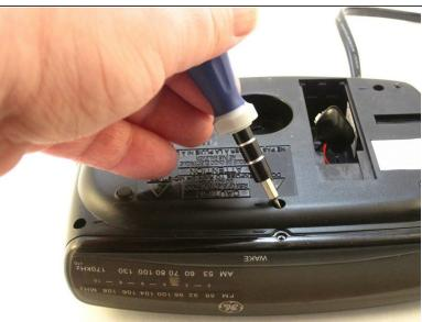
Using a Phillips #00 Screwdriver, unscrew the six 12mm screws from around the bottom of the clock radio.
