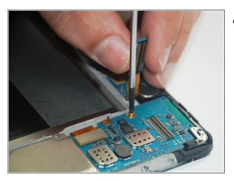
Remove the screws securing the flex cable to the chassis.
