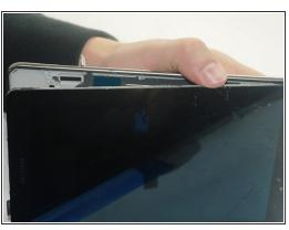
Using the prying tool, pry the silver binding from around tablet from glass edge. You will need to go around the device several times applying some force before it comes off.
