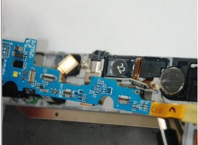
Remove the original flex cable and replace it with the flex cable.
