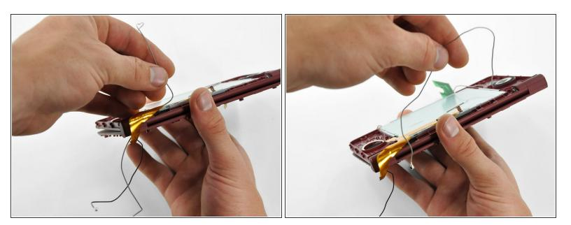
Pull the Wi-Fi antenna cable through the right hinge connecting the front bezel and upper case.
