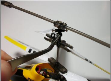
Using tweezers, gently remove the two stabilizing links by pulling straight away from the point of connection.
