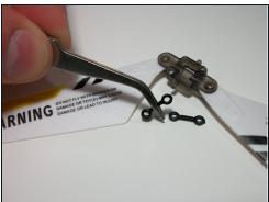
• Again using tweezers gently remove the stabilizing links from the blade carriage by pulling straight away from the point of connection.
