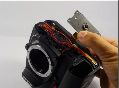
Carefully wiggle the yellow metal tab to remove the plate.
