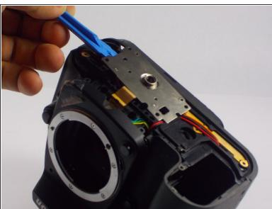
Now use a plastic opening tool and carefully pop off the metal tripod thread plate.
