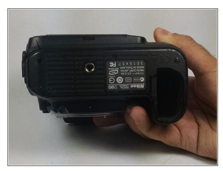
• Turn the camera so the bottom casing is facing up.
