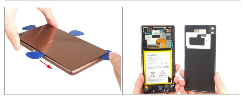
• Slide the guitar pick to cut the sticker and remove the back cover.
