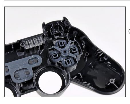
The D-pad has a three-armed plastic piece that must be installed as shown before installing the rubber button pad for it to work properly.
