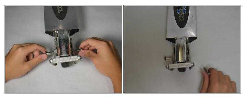
• Remove the bolt from the right side and the bearing from the left.
