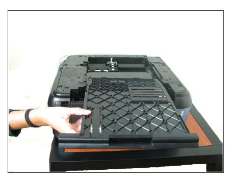
Firmly grasp the tray and remove from rest of the printer.
