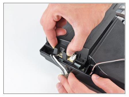
• Lift the power supply upward from its left edge as viewed from the front of the PS3.
