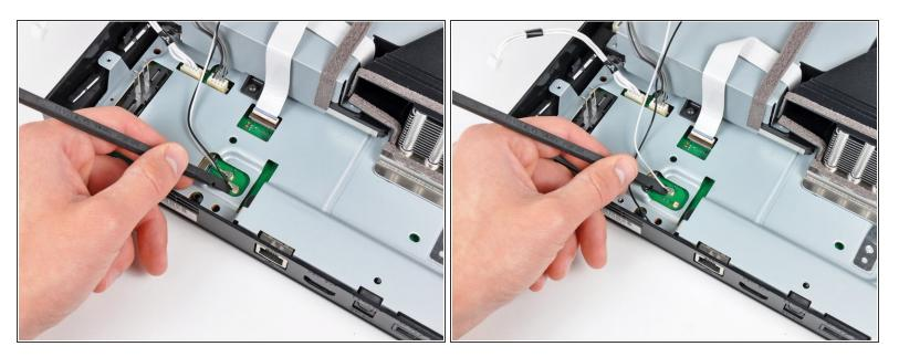
Use the flat end of a spudger to pry both antenna connectors up off their sockets on the motherboard.
