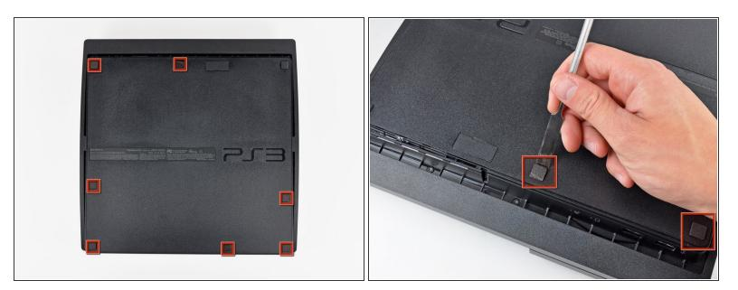
Use the flat end of a metal spudger to pry up the seven screw covers around the edge of the lower case.
