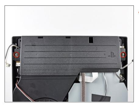
Remove the two 7.6 mm Phillips screws securing the power supply to the lower case.
