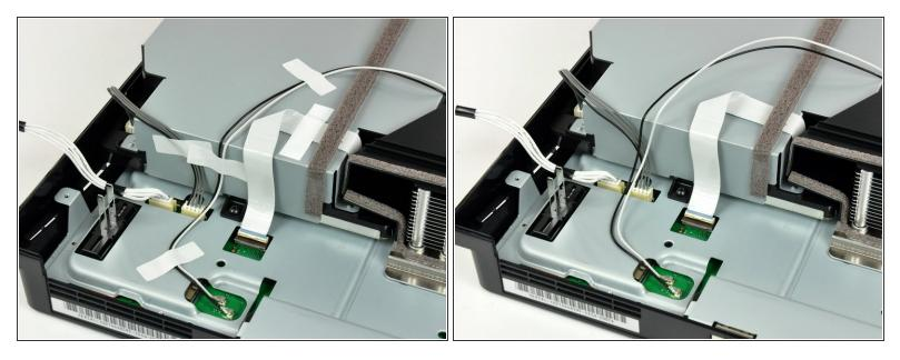
If present, remove the pieces of tape securing the antenna cables to the fan shroud, Blu-ray drive, and top shield.
