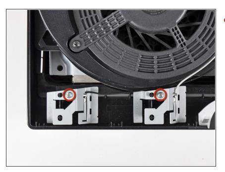
Remove the two 6.2 mm Phillips screws securing the antennas to the lower case.
