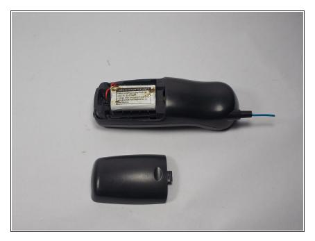
To remove the battery cover, push in and downwards towards yourself on the cover. There is a notch on the back that you can use to get a better grip if necessary.
