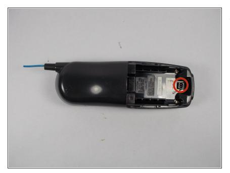
Pull the battery away from the battery housing. At the end of the wires on the housing side there is a clip that connects the battery to the phone. Unplug this clip and discard the warn battery appropriately.
