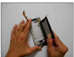
• Use a wide pry tool or credit card to gently pry the battery up and out of the phone.
