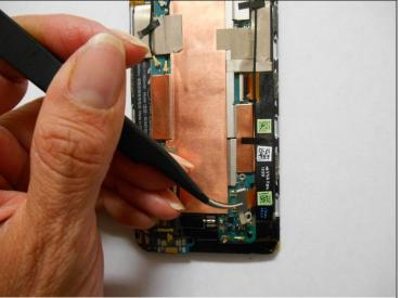
• Disconnect the battery by prying the metal cover straight up.
