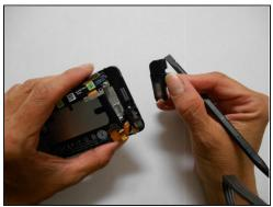
Using the spudger, use force to detach and remove the speaker.
