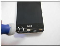
• Remove the screw under the speaker cover using a T6 Torx screwdriver.
