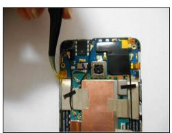
• Use <u>tweezers</u> to remove the yellow tape covering the flex cable connectors (total of five).
