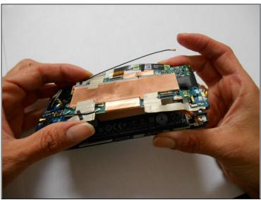
• Lift the motherboard, but don't try to remove it completely yet.
