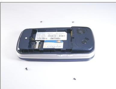
Use a Phillips screwdriver to remove the four 2mm Phillips #000 screws from each corner of the device.
