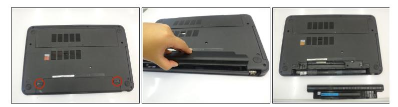
We are removing the battery to avoid the possibility of an electrical discharge when working with this system.
