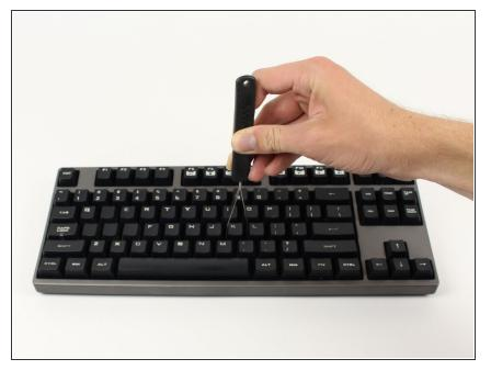
Insert the keycap puller around the key you want to remove.
