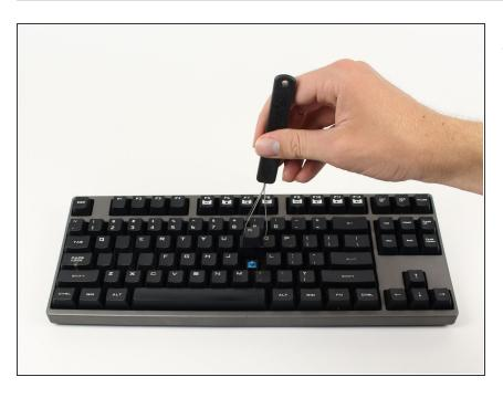
• Pull cap directly upward.
