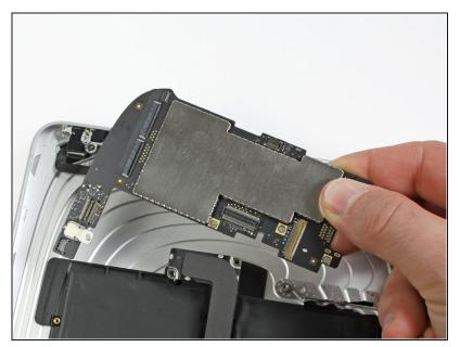
• Lift the logic board out of the rear panel assembly.
