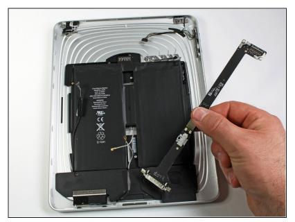
• Lift the dock connector cable out of the rear panel assembly.
