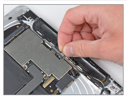
Pull the GPS antenna ribbon cable out of its socket.
