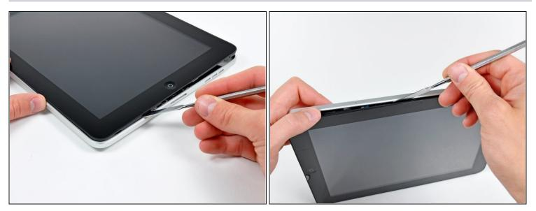
• Continue prying the display assembly away from the rear panel along the bottom and left edges of the iPad.
