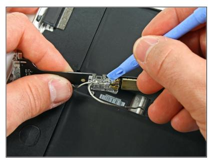
Using an iPod opening tool, carefully remove the plastic cover shielding the WiFi/Bluetooth board and dock connector cable.
