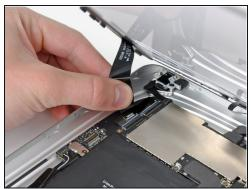
• Use the edge of an iPod opening tool to flip up the retaining flaps holding the digitizer ribbon cables in their sockets on the logic board.
