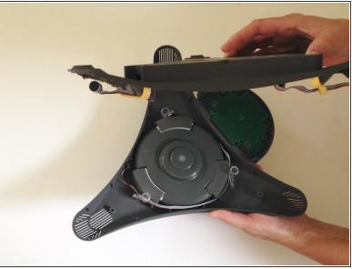
Gently lift and separate the back housing from the rest of the device. Now you've got the back housing off!
