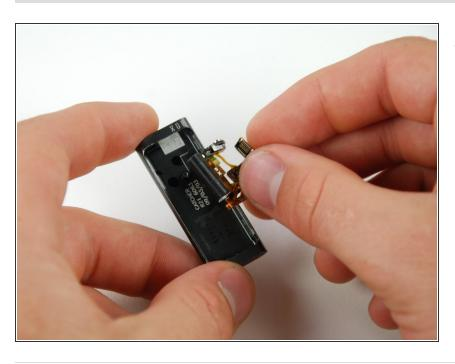
Remove the headphone jack and shuffle switch from the front case.
