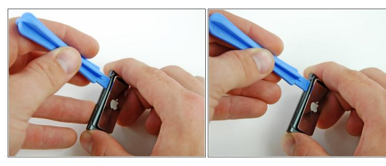
Insert an iPod opening tool into the newly widened gap, and pry the rear case up and away from the front case.
