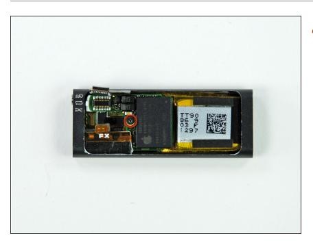
Remove the single Phillips screw securing the logic board to the front case.
