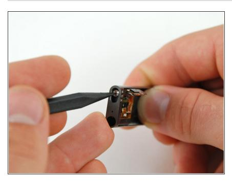
Using the pointed tip of a spudger, push the shuffle switch in to separate it from the front case.
