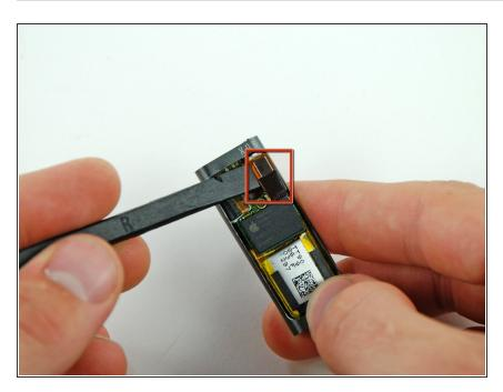
Disconnect the headphone jack and shuffle switch connector by prying it off the logic board with a spudger.
