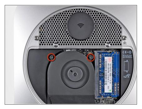
Remove the two 11.3 mm T6 Torx screws securing the fan to the logic board near the antenna plate.
