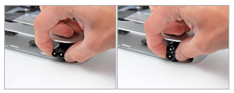
• Rotate the AC-In connector 90 degrees counter-clockwise.
