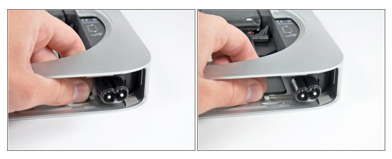
• Pull the silver metal AC-In socket retainer away from the side of the outer case and remove it from the mini.
