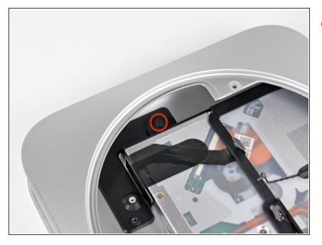
Remove the 7.9 mm T6 Torx screw securing the optical drive to the outer case.
