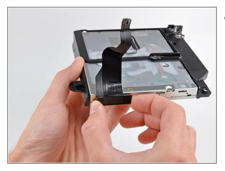
Remove the optical drive cable by pulling its connector away from the body of the optical drive.
