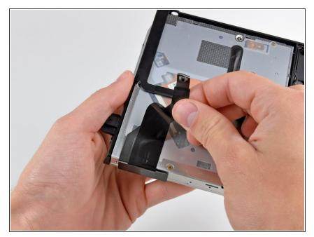
• Peel the optical drive cable off the body of the optical drive.
