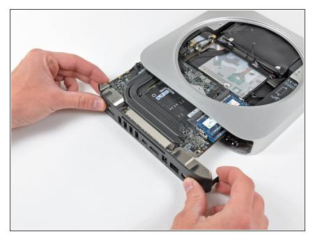
Carefully slide the logic board assembly out of the mini, minding any cables that may get caught.
