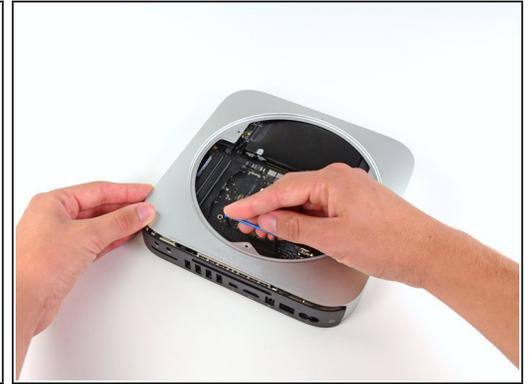
**i** For enough clearance to remove the hard drive, the logic board must be slightly removed. To accomplish this, two cylindrical rods must be inserted into the holes highlighted in red.
