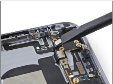
• Use the flat end of a spudger to lift the volume control cable connector up off of its socket.
