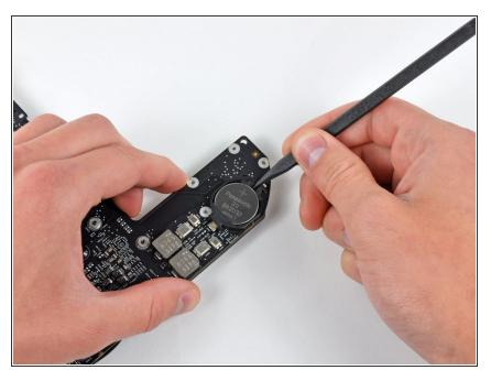
Use the tip of a spudger to carefully pry the PRAM battery up and out of its holder on the logic board.
