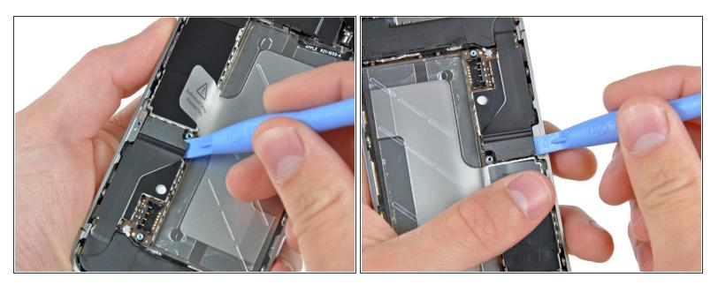
Use an iPod opening tool to gently pry the dock cable connector up off the logic board from both short ends of the connector.
