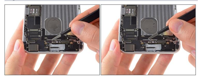
• Grasp the antenna connector with a pair of tweezers and gently lift it from its retaining clip on the logic board.
