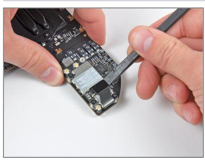
Use the flat end of a spudger to pry the AirPort/Bluetooth ribbon cable connector up off the AirPort/Bluetooth board.
