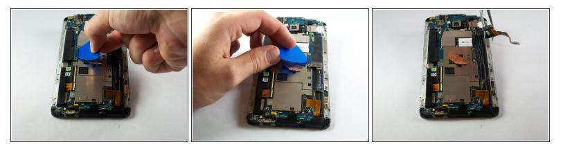
Use a plastic tool to pry up and disconnect the large ribbon cables on each side of the motherboard.
