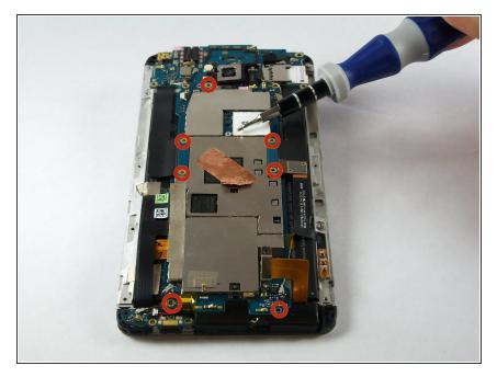
Remove the seven 3 mm Phillips #000 screws from the motherboard.
