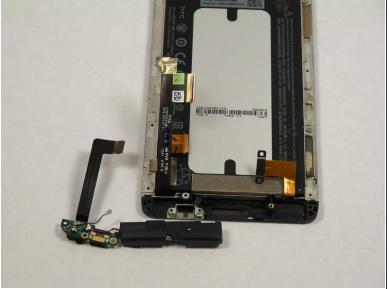
Use the small plastic opening tool to pry back the speaker and microphone assembly from the bottom of the phone.
