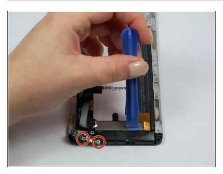
Remove the two 2.8 mm Phillips #000 screws from the metal plate near the bottom of the phone.
