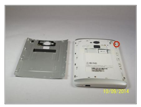
Lift back cover while pressing highlighted release switch towards the center of the phone.
