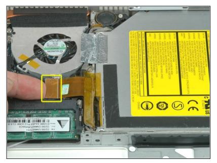
• Disconnect the orange optical drive ribbon cable from the logic board.
