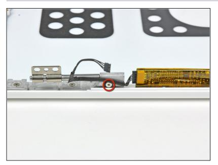
• Remove the single 3.2 mm Phillips screw securing the inverter cable to the left clutch hinge.
