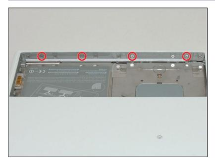
Remove the four 3 mm indicated Phillips #00 screws from the front wall of the battery compartment. When working from the left, remove the 2nd, 4th, 7th and 9th screw.
