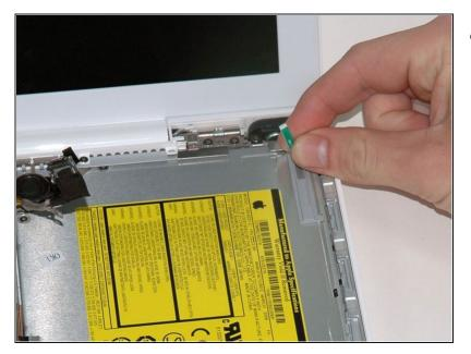
• Lift the Bluetooth antenna board from the right side of the optical drive.
