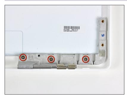
Remove the three 3.2 mm Phillips screws securing the right clutch hinge to the rear display bezel.
