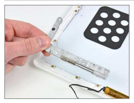
• Remove the left clutch hinge from the rear display bezel.
