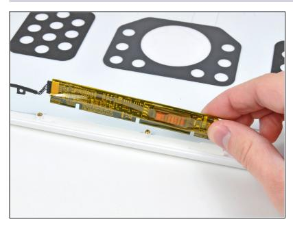
• Remove the display inverter and its attached cable from the rear display bezel.
