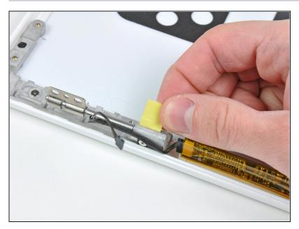
• Remove the piece of tape stuck to the left clutch hinge.
